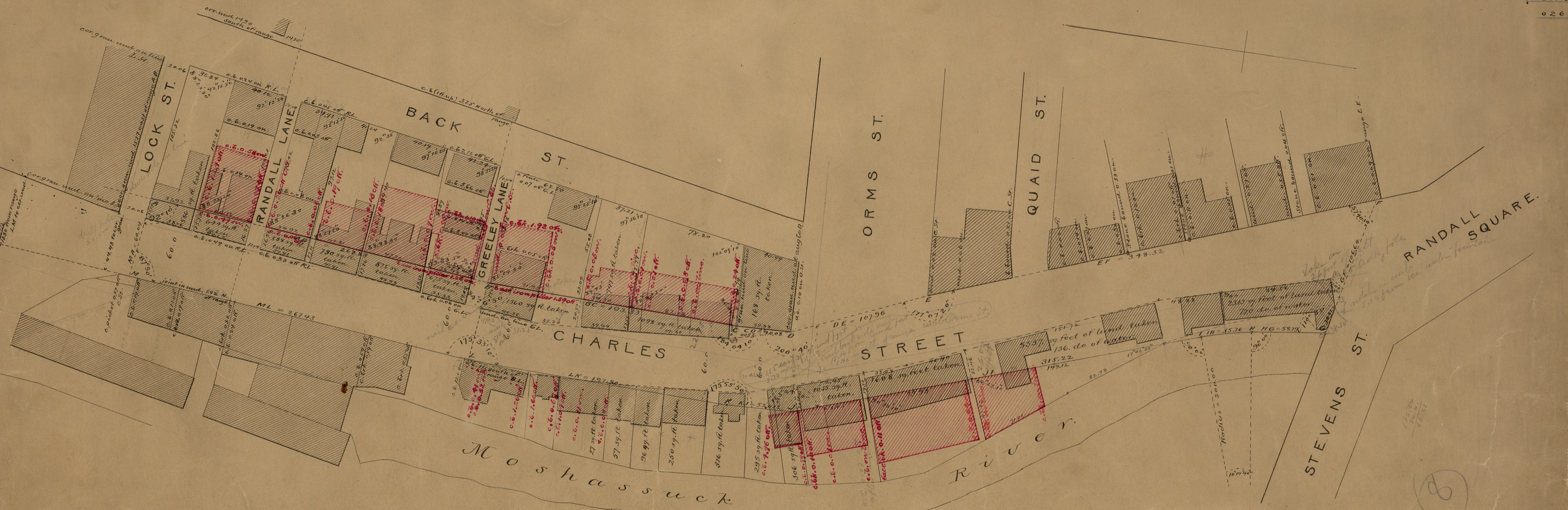
Map showing widening of Charles Street from Lock Street to Randall Square. Scale 40 feet per inch.
